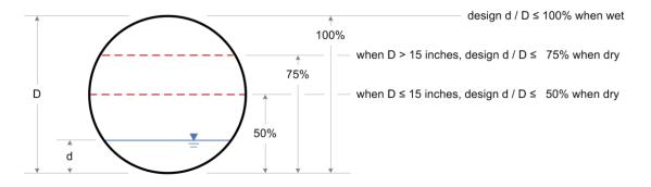
The authors have used such guidelines as KPIs for a number of years to evaluate existing sewer systems under actual operating conditions, and the results can be presented and explored in graphical form as shown in Figure 2. This graphical method evaluates expected maximum hourly average flow depth data within existing sewers in the context of ASCE and WEF sewer design guidance. It can also be adapted to reflect local sewer design requirements, as needed.
