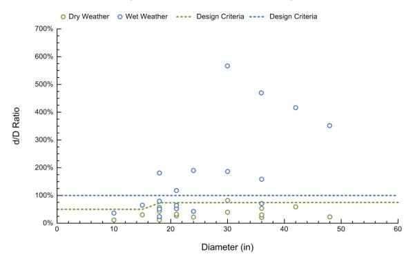
FIGURE 2: Evaluating Sewer Performance in Context of Sewer Design Guidance
