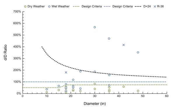
FIGURE 6: Evaluating Sewer Performance in Context of Capacity Assurance Criteria
